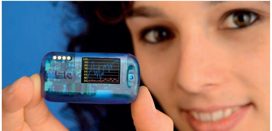
Wireless monitoring of measured data and fast readings of measured values – the new features of the Bluetooth Low Energy Option and the OLED graphic display of the MSR145 mini data logger. Also new: the web-based “MSR SmartCloud” service for mobile data monitoring.
