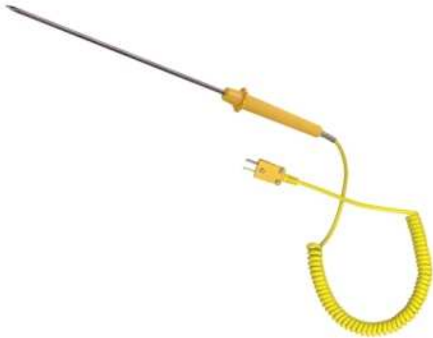
ATT50 Immersion K-Type Temperature Probe 8 inch for Liquids with Handle and Pointed tip. Range : -40°C ~ 850 °C
