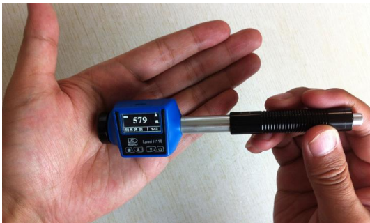
Leeb hardness measurement principle
