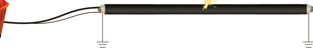
High resistance fault in cable's intermediate joint being burn through
