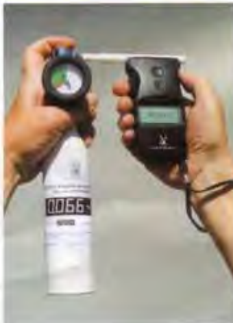
The Lion Alcolimeter 500 being calibrated with a Lion AlcoCal S alcohol calibration standard
