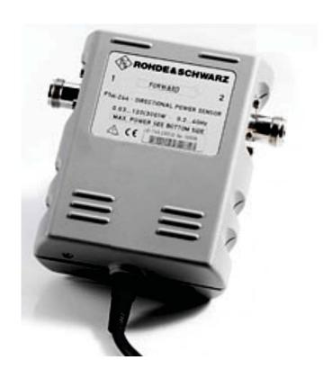
The R&S°FSH-Z44 Directional Power Sensor is to be used with the R&S°FSH handheld spectrum analyzer for simultaneous measurement of forward and reflected power. The R&S°FSH-Z44 offers a frequency range from 200 MHz to 4 GHz and a measurement range from 30 mW to 120 W. (300W with Unmodulated Envelope)
