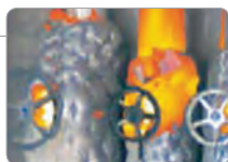
Fused thermal images insert IR image set within a temperature interval onto corresponding digital image
