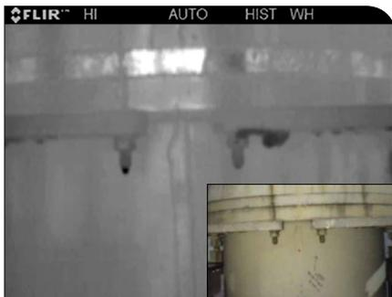
Visible vs. OGI image of SF<sub>6</sub> leak
