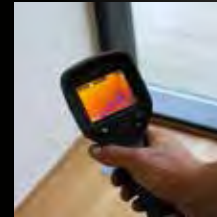
Find air infiltration problems
