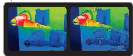
Original IR Image on the Left and with MSX™ Enhancement on the Right image (available on T640 model)
