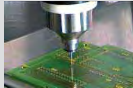
Centering unit for pinpoint cell positioning on small areas
